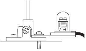
WindTrak Light with **WindTrak 10** (#3120) or **J-Base** mounting sockets (#3125, #3155).
