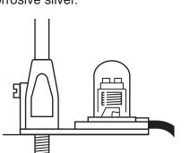
WindTrak Light with **WindTrak 15** (#3150). Mounts directly on the threaded part of the mounting sockets.
